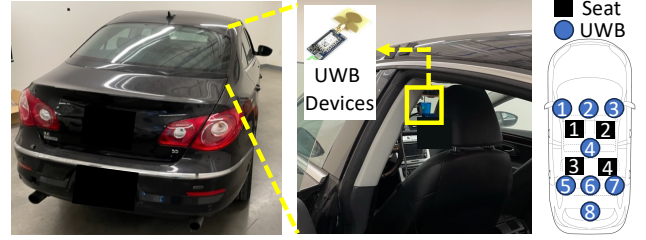
Figure 15: UMusic leverages the UWB devices deployed to the eight locations inside a sedan parked in a garage.
